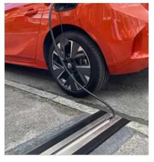
Comments: Currently undergoing public trials within Shropshire LA. This unit removes the risks associated with the gully gap permanently left open at the
